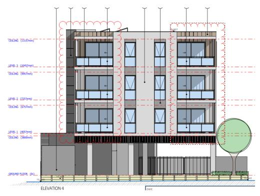
Figure 3 – Extract of the rear elevation showing the proposed balcony areas (clouded in red)
