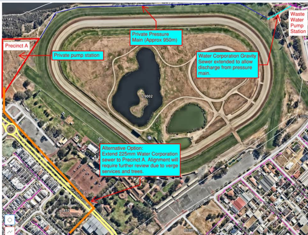
Figure 9 – Existing Gravity Wastewater Reticulation Services (Water Corporation)
