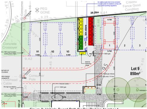
Figure 3: Vehicle Swept Path for Car Parking Number 1
