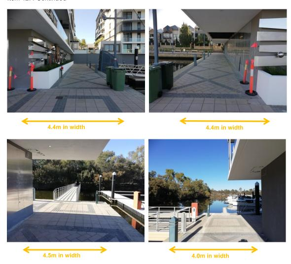
Figure 6: Remaining width of pedestrian area once artwork has been installed
