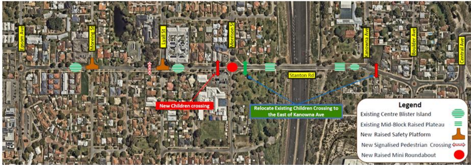
Figure 11: Existing and proposed traffic calming measure along Stanton Road and Second Street
