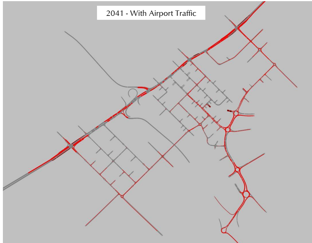
Figure 13: Snap shot of VISSIM PM model – 2041 with Perth Airport West Precinct traffic generation
