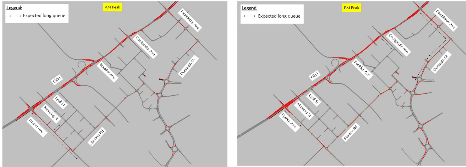
Figure 9: VISSIM modelling output for closure Moreing Street, Lyall Street and Boulder Avenue at GEH
