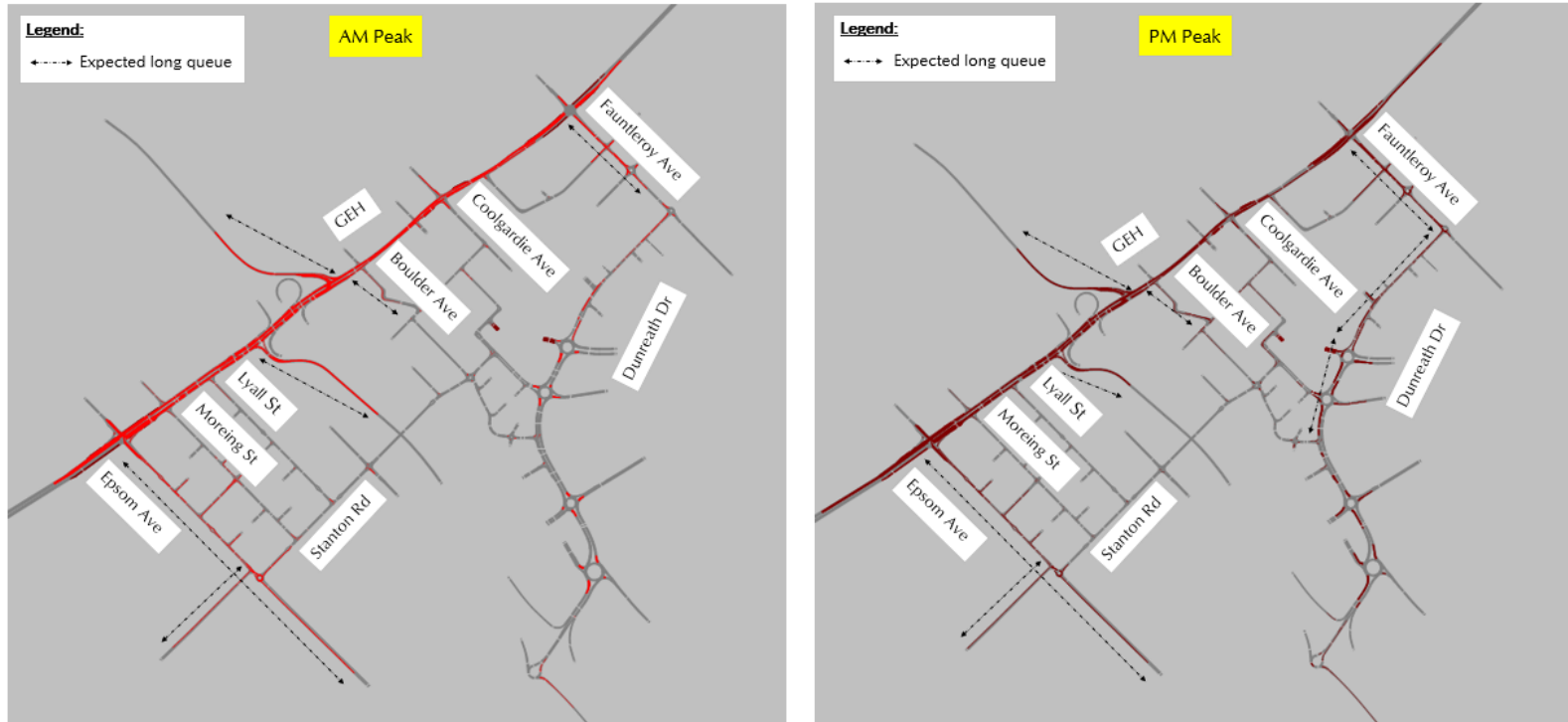
Figure 8: VISSIM modelling output for closure of Stanton bridge
