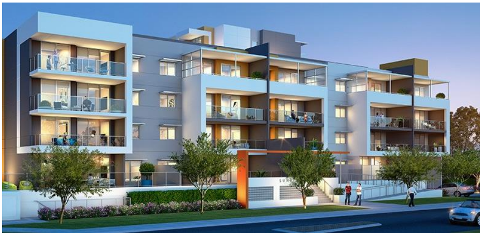
Above: Example of a 4 storey residential building detailing an appropriate level of articulation and surveillance through the use of balconies and architectural elements. Also illustrates an acceptable treatment to site retaining at lot edges.
