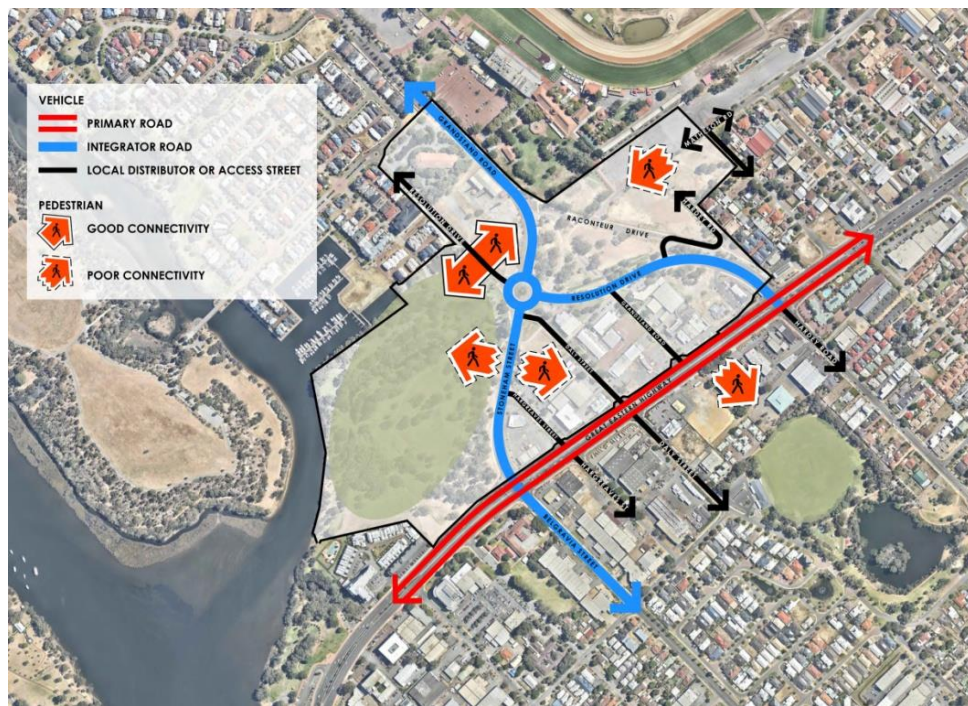
Figure 10 - Existing access and connectivity summary
