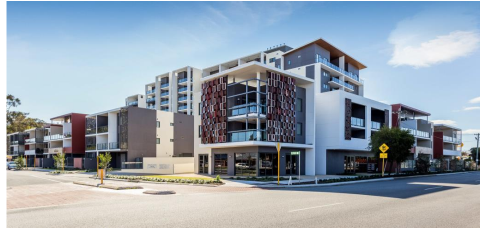
Above: Corner site development addressing both street frontages, with 3 storey podium height to building edges and mixed height elsewhere on site.
