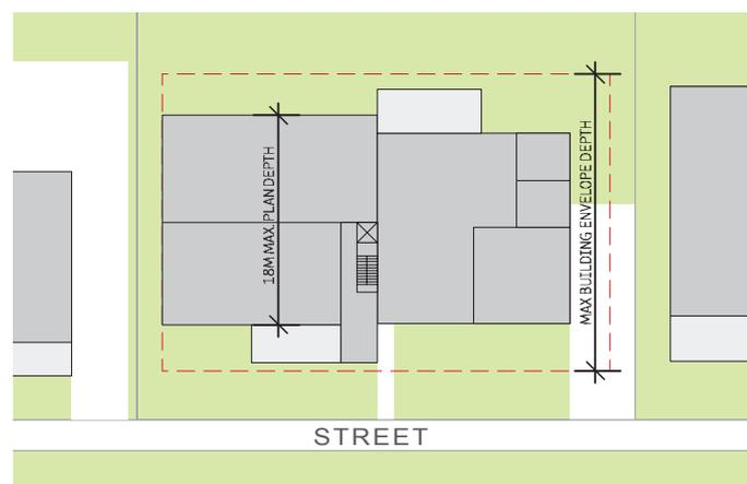
FIGURE 3.1.2: DIAGRAM 4: PLAN DEPTH TO BE NO GREATER THAN 18M GLASS LINE-TO-GLASS LINE IN RESIDENTIAL BUILDINGS STREET
