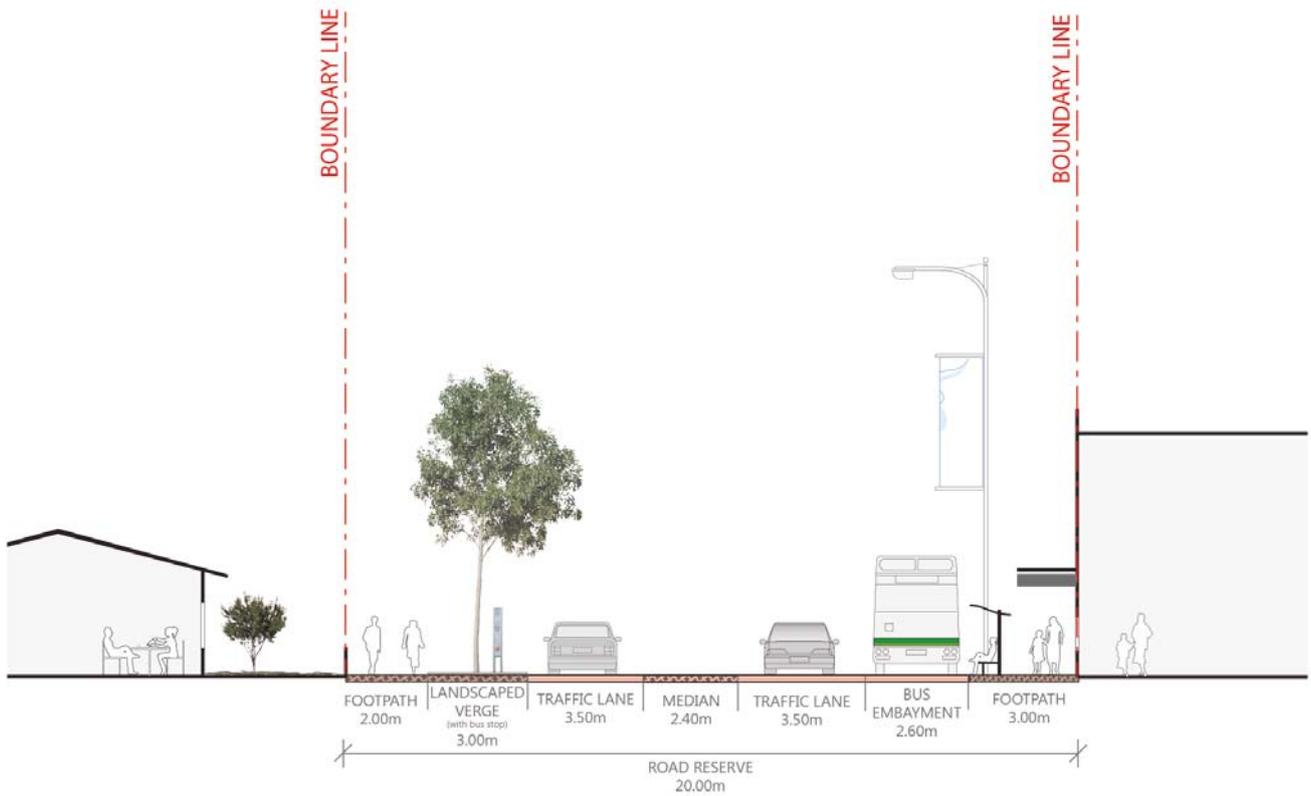
Figure 14: Cross Section CC - Relocated Supermarket fronting Belvidere Main Street
