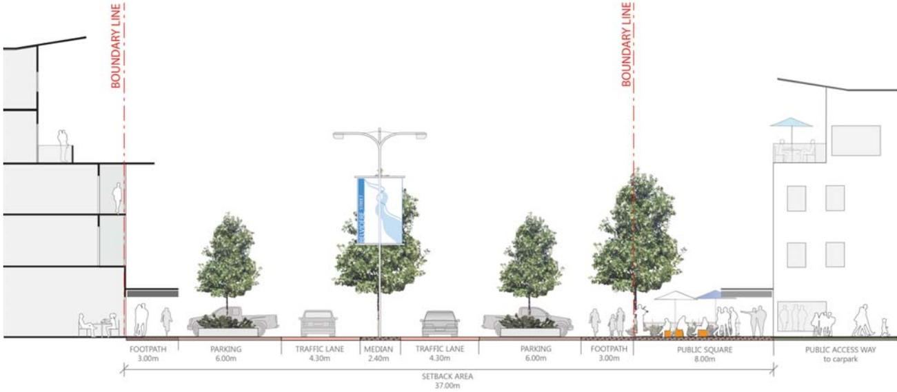
**Figure 8:** Cross Section BB: Belvidere Main Street
