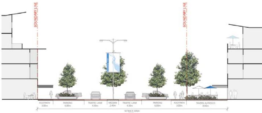
Figure 15: Cross Section DD - Relocated Tavern fronting Belvidere Main Street
