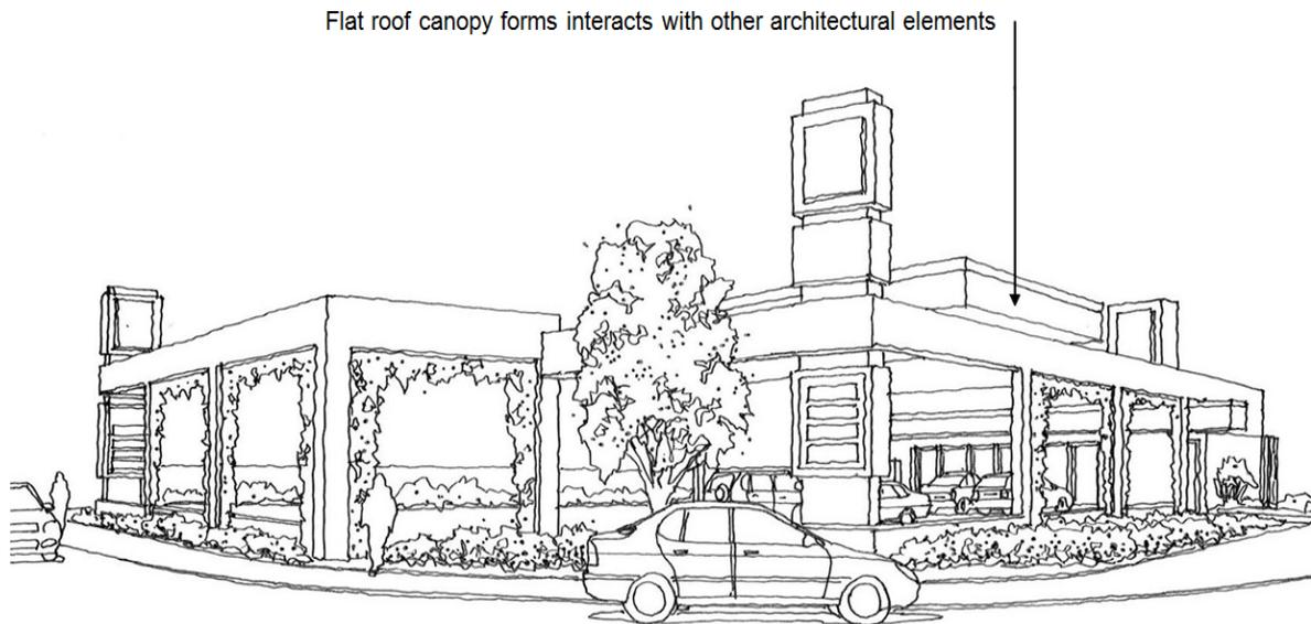
Figure 4 - Flat roof canopy design integrated into an overall architectural composition of buildings, screen walls, pylons and other elements.
