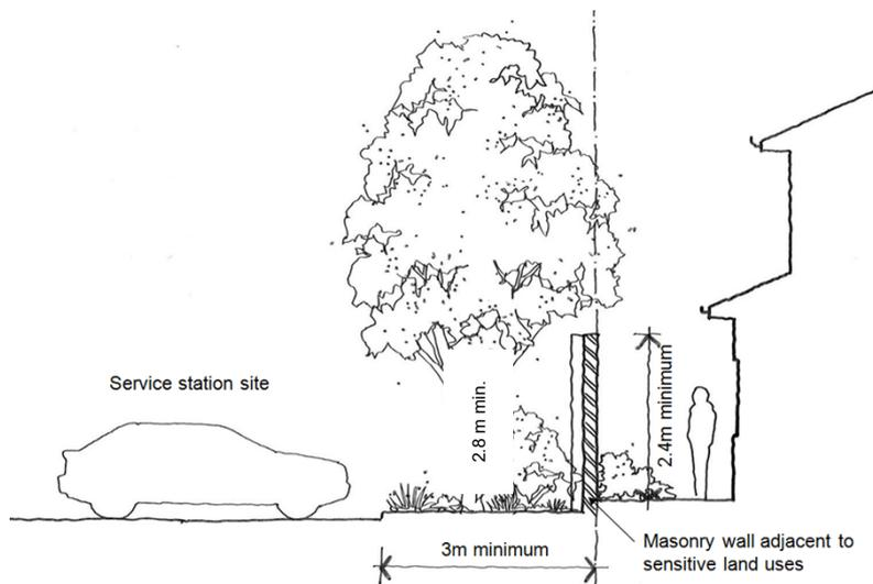
Figure 7 - An appropriate boundary treatment with landscaping and a masonry wall.
