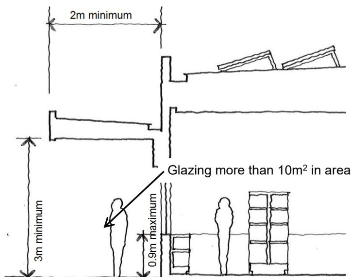
Figure 5 - Appropriate building interface with glazing and an awning for shade and shelter.
