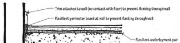
Figure 2.1: Floor acoustic decoupling example construction
