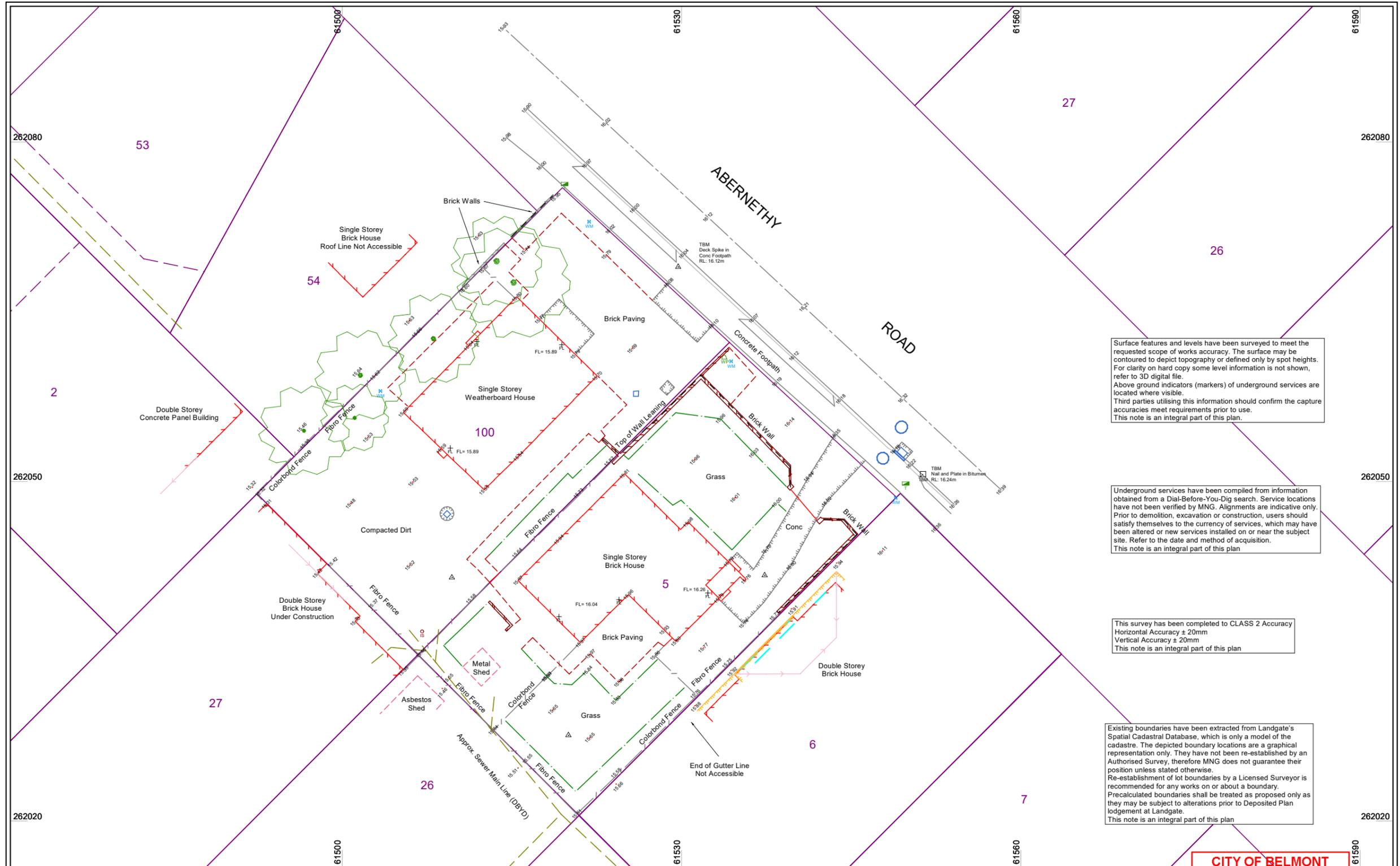
Surface features and levels have been surveyed to meet the requested scope of works accuracy. The surface may be contoured to depict topography or defined only by spot heights. For clarity on hard copy some level information is not shown, refer to 3D digital file.
