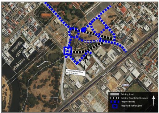
Figure 24: Proposed Grandstand Road realignment and extension
