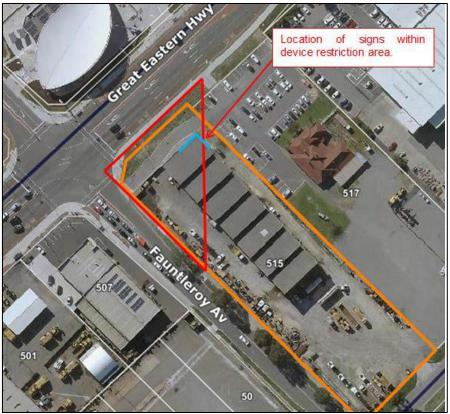
Figure 6 - Approximate location of signs with Device Restriction Area
