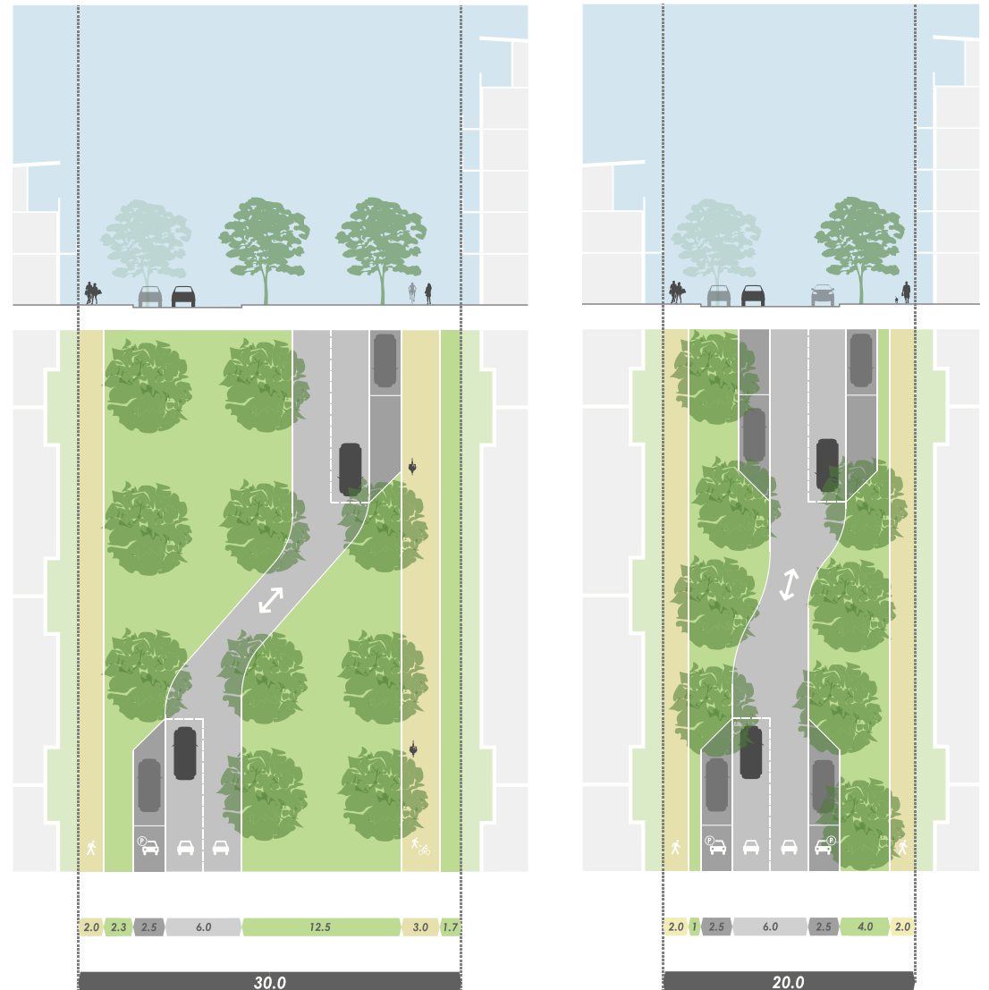
Figure 33: Concept design for road upgrades for identified 'Street Character Type C' roads.
