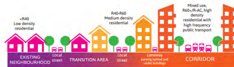
Figure 3 Cross Section Illustrating Proposed Interface from Corridors to Neighbourhood Area (Perth and Peel @ 3.5 Million)
